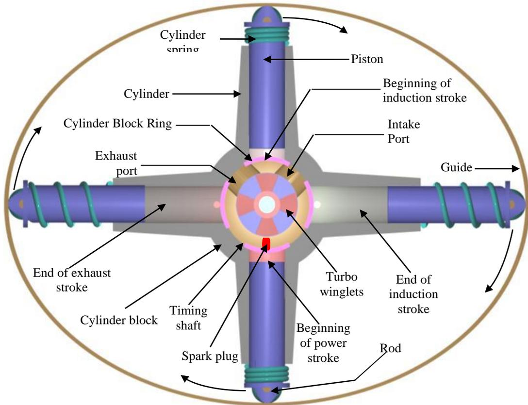
Figure 3.1. Cutaway view of elliptic engine
