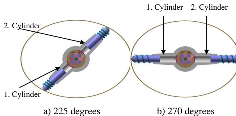
Figure 3.5. Operational Principle of Elliptic Engine Third Period (225-270 degrees)
