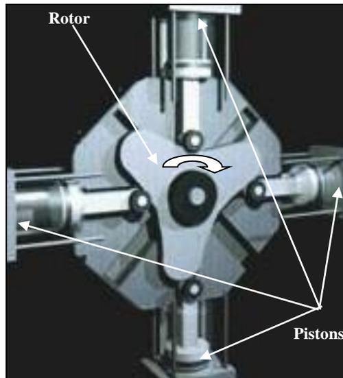
Figure 2.1. The General View and Operation of the Tritec Engine
