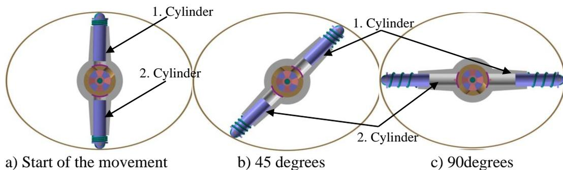
Figure 3.3. Operational Principle of the Elliptic Engine, First Period (0-90 degrees)
