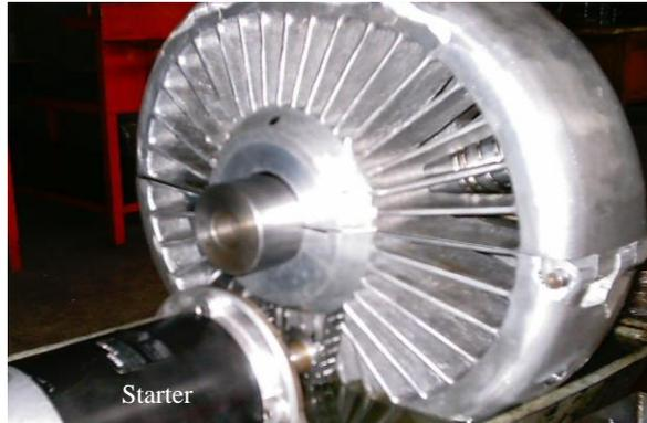
Figure 4.1. First installation of the elliptic engine (closed body)
