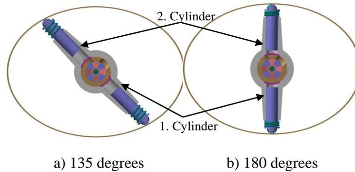
Figure 3.4. Operational Principle of the Elliptic Engine, Second Period (135-180 degrees)
