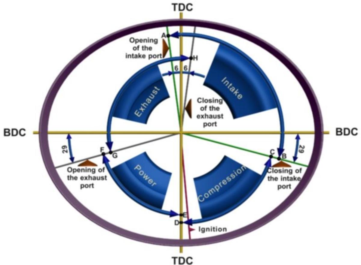
Figure 3.7. The valve timing diagram of the elliptic engine
