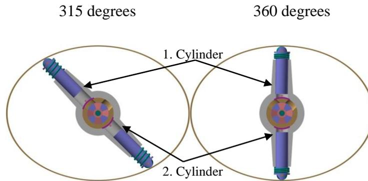
Figure 3.6. Operational Principle of Elliptic Engine Fourth Period (315-360 degrees)
