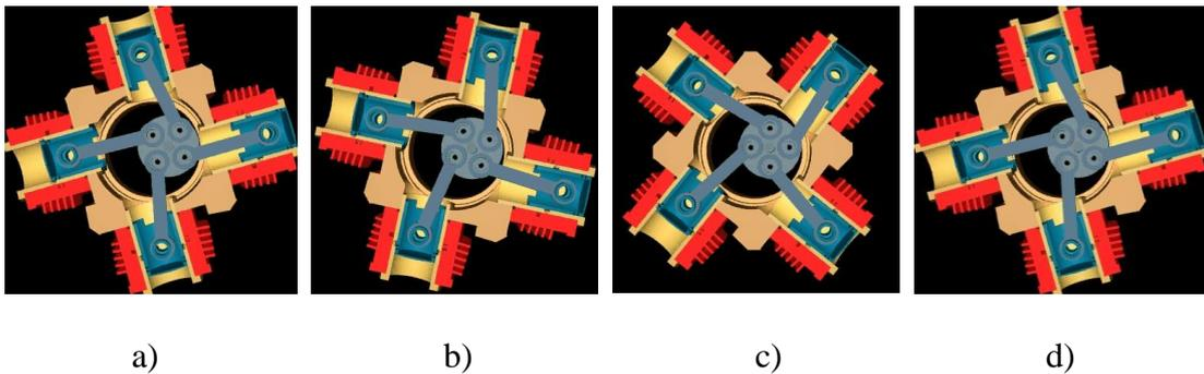
Figure 2.4. Operation of Rotary Body Markel Engine
