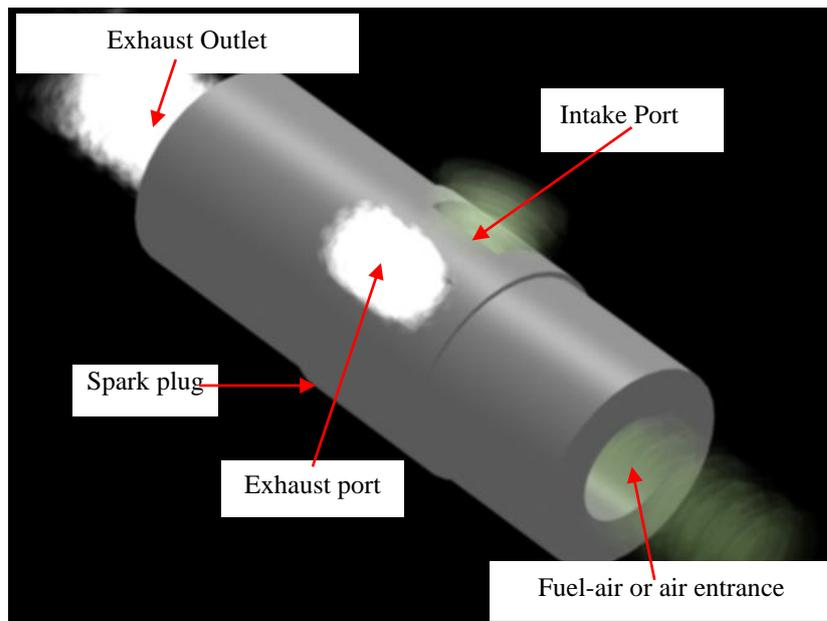
Figure 3.2. Timing shaft and parts of the Elliptic Engine
